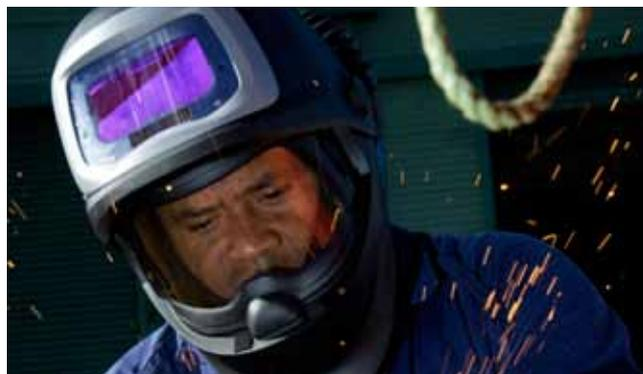
All the benefits of the Speedglas welding helmet 9100 FX can now be used in conjunction with head protection (AS/NZS1801) for welders working in areas with overhead hazards.
